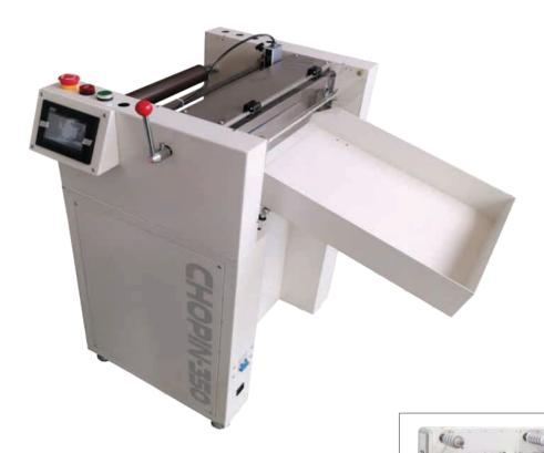
CHOPIN 350 is an optional sheeter for digital roll die-cutting machine. CHOPIN 350 runs in connection with DUOBLADE SX inline. Speed of each machine is synchronized by data signal communication.
